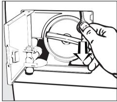
■ To open the door, pull down on the ring in the upper right corner of the access area.
